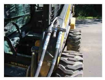
Figure 33: Hydraulic Lines Connecting to Skid Steer from Road Widener
