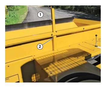
Figure 26: Tailgate Stop Bar, Clevis Pin and Clip
