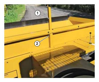
Figure 34: Tailgate Stop Bar, Clevis Pin and Clip
