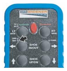
Figure 29: Amber Battery Status LED
