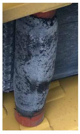
Figure 43: Material Buildup
