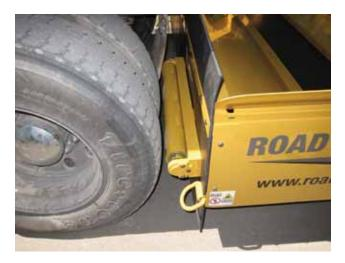
Figure 39: Rollers Touching Truck Wheels
