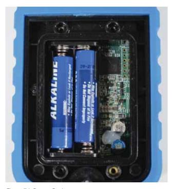
Figure 74: Battery Replacement
