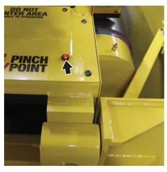
Figure 32: Blinking Red LED Light
