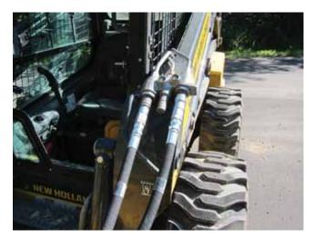
Figure 24: Hydraulic Lines Connecting to Skid Steer from Road Widener
