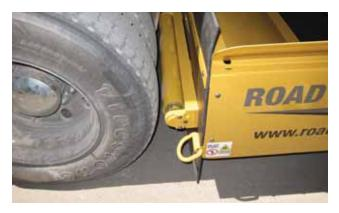
Figure 54: Rollers Touching Truck Wheels
