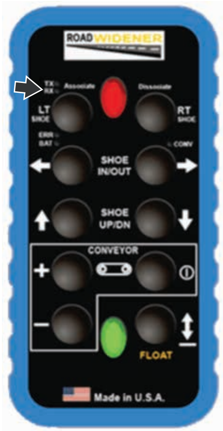
Figure 82: TX and RX LEDs Flashing
