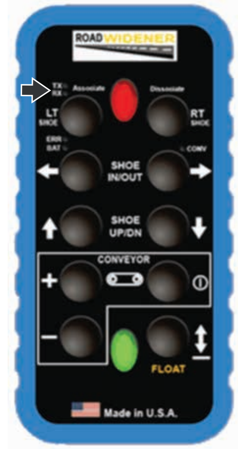
Figure 78: TX and RX LEDs Flashing
