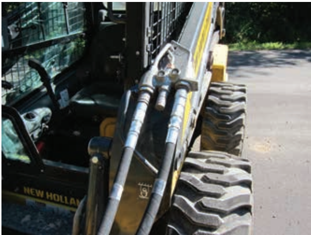
Figure 25: Hydraulic Lines Connecting to Skid Steer from Road Widener
